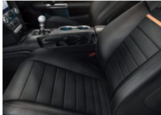
Seat insert: Register Enhanced Mini Perf over Luxury Grain Leather in Ebony with Orange accent stripe Bolster: Lux Grain Vinyl in Ebony with Metal Grey contrast stitching
